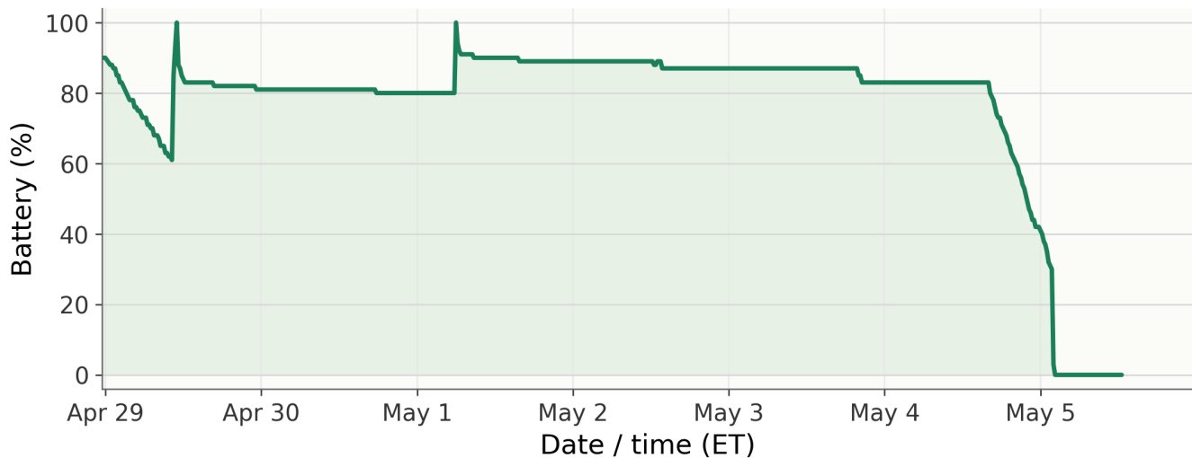
Figure 4.1. Thingy internal battery during the one-week outdoor deployment. The trace shows the battery telemetry recorded from Apr 28 to May 5, 2026 ET under the continuous-post firmware; it reflects the Thingy internal battery, not direct external 10 Ah buffer state of charge.
