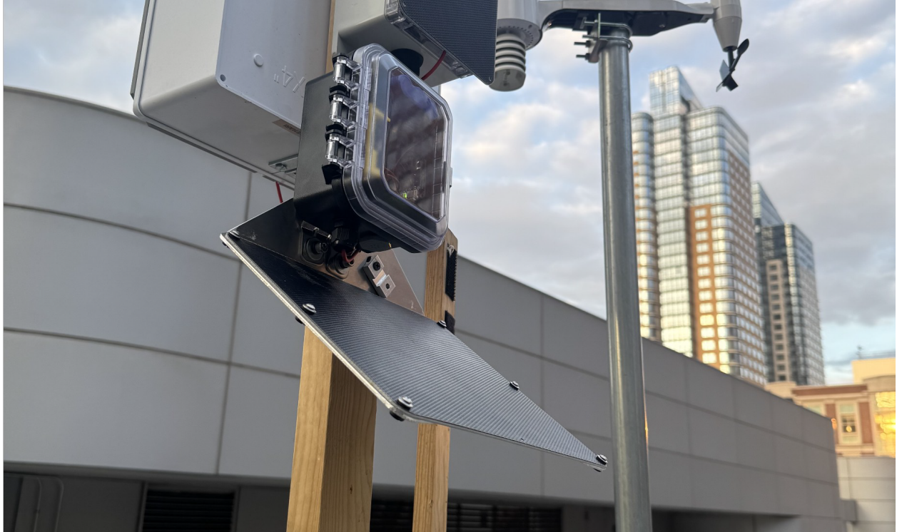
Figure 3.2. Assembled prototype hardware used for integration testing. The photo shows the physical sensor node, solar panel, and external power hardware in the outdoor test configuration used before final tower-rated enclosure and rigid PR tower mounting are completed.
